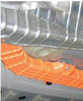
*Electrical shield bolted to undercarriage*
