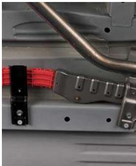
*Thermal shield near hot exhaust*
