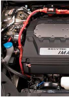
*High-Voltage Cable to Accord AC Compressor*
