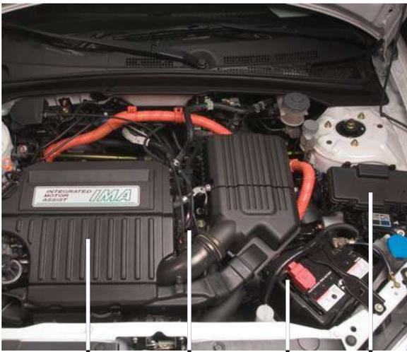
Engine      Motor      12-Volt Battery      Underhood Fuse Box
