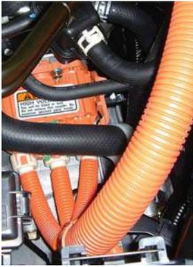
*High-Voltage Cable Connection to Motor*
