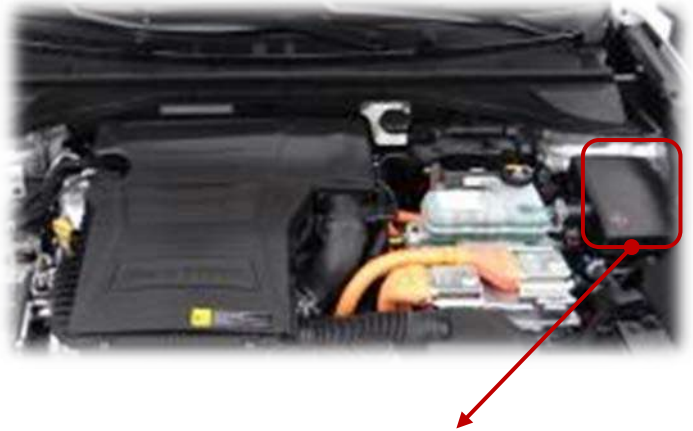
Engine room fuse box
