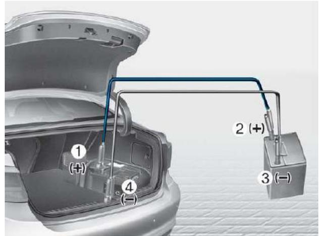
Proceed to connect one end of the other jumper cable to the negative terminal of the booster battery, then the other end to a solid, stationary, metallic point away from the battery (for example, the tailgate latch).
