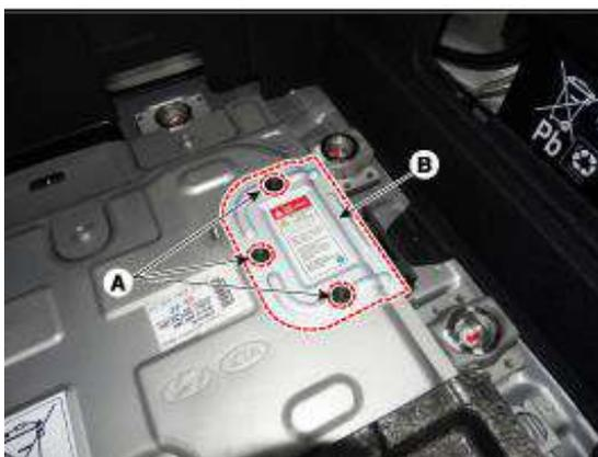
A: Unlock → B: Release → C: Remove
