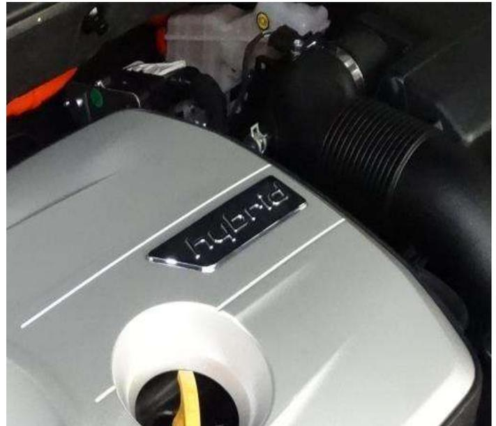
Additionally, there are orange colored high-voltage electrical cables in the engine compartment.
