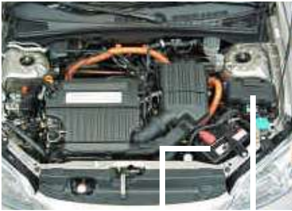
12 V Battery Under-hood Fuse Box
