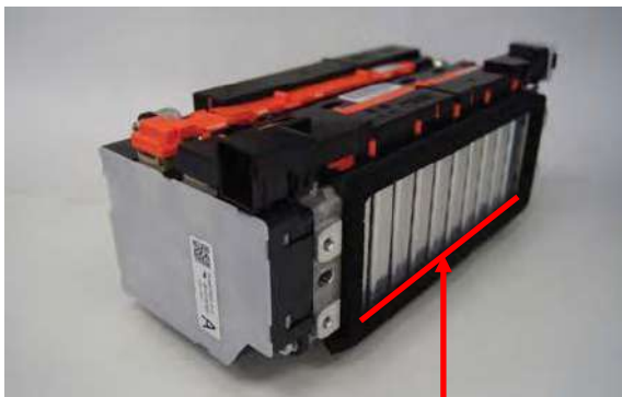
One of Four Battery "Stacks"
