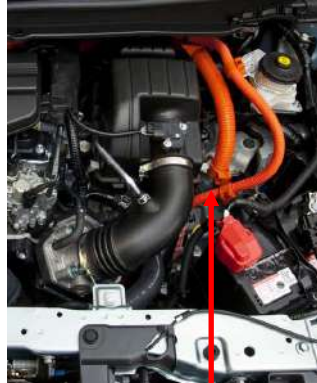
High-Voltage Cord to Civic AC Compressor
