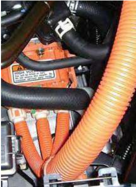
High-Voltage Cable Connection to Motor
