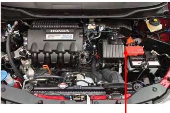
Positive Battery Terminal
