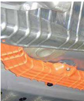
Electrical shield bolted to undercarriage
