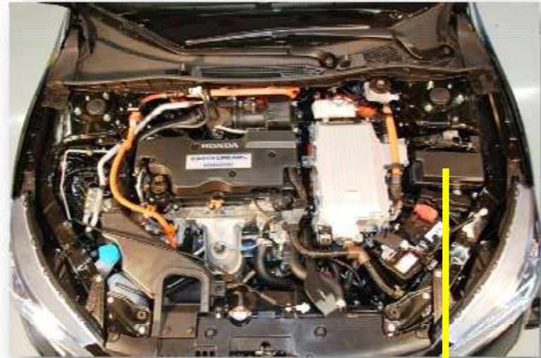
Underhood Fuse Box
