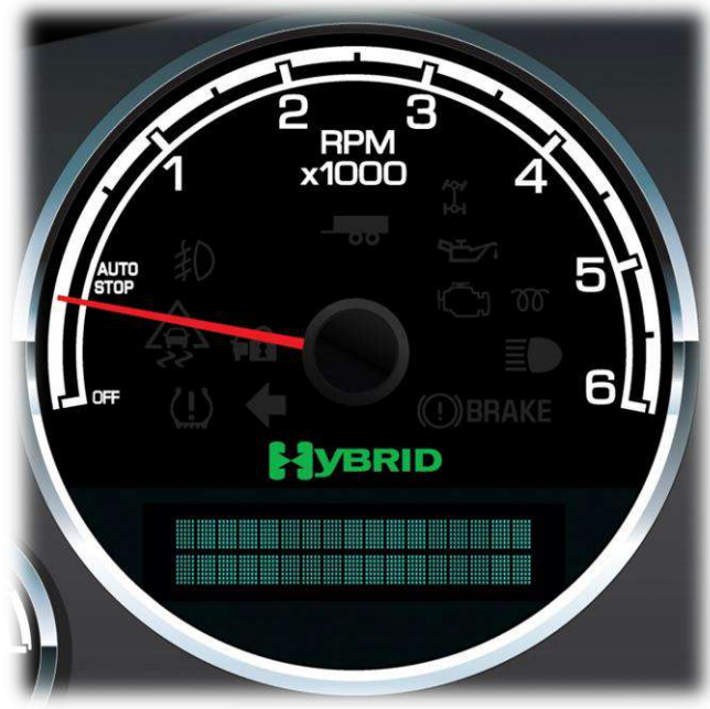
Tachometer with Auto Stop Indicator
