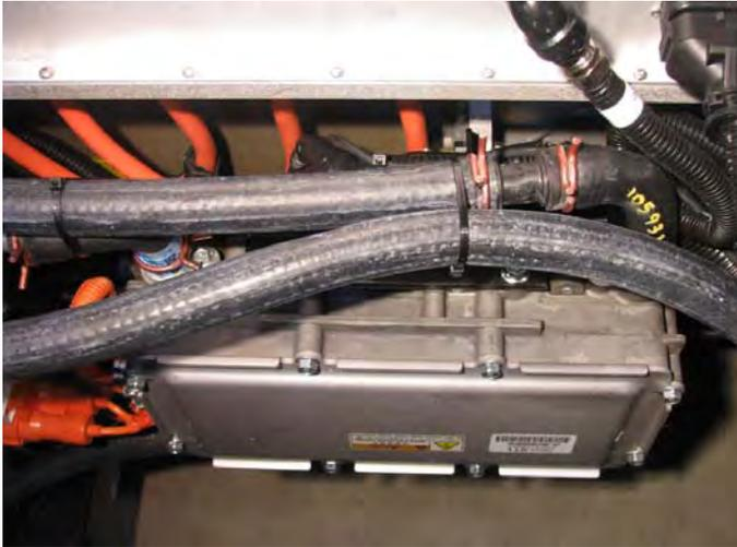
Orange cabling is found under the hood and underneath the vehicle to identify those wires carrying high voltage.
