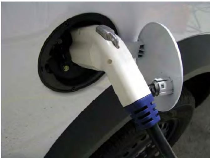
On the Right side of the vehicle – in the area normally occupied by the fuel cap – is the charge port.
