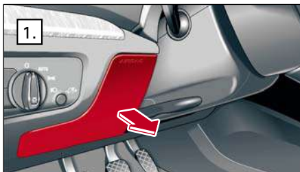
Fuse box – left-hand drive (steering wheel left)
