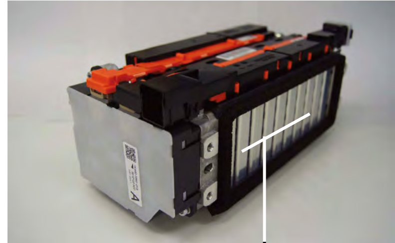
One of Four Battery “Stacks”
