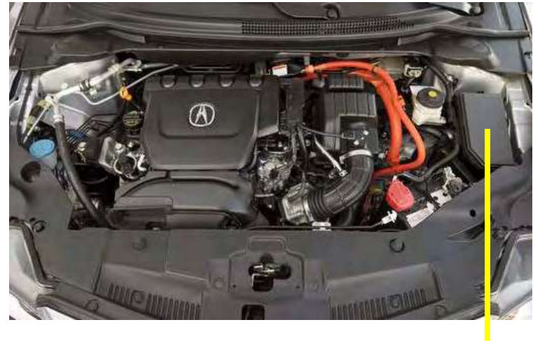
Underhood Fuse Box
